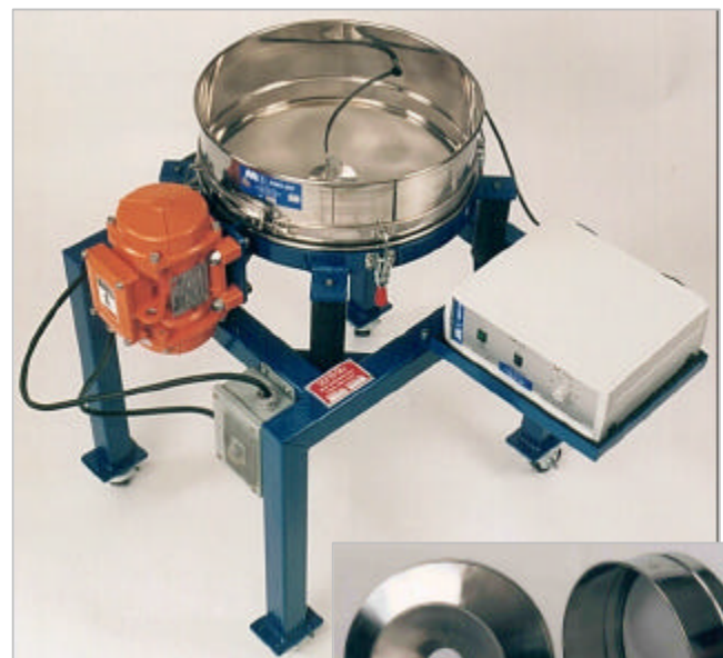
Model RVM-15E with SFA Ultra-sonic kit.
